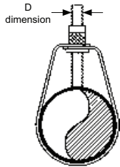
Adjustable swivel Ring - rod tight to pipe
