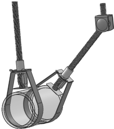
BRANCH LINE RESTRAINT NFPA13 2010 Section A.9.3.6.1(5)
