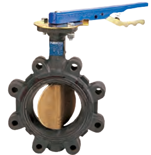
LD-3100 Lug Style Buna-N Liner and Aluminum Bronze Disc
