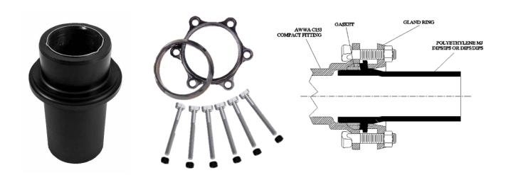
The MJ Adapter is a polyethylene fitting that is designed to; a) make a transition to or from a non-polyethylene system by use of a standard ANSI/AWWA mechanical joint, or b) give you the ability to connect a polyethylene system to traditional hydrants, valves, and metal pipes using a standard ANSI/AWWA mechanical joint fitting.
