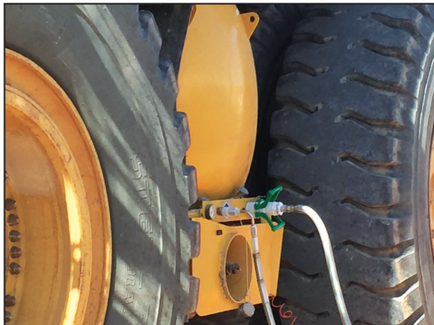
LNG fueling application on off-highway mining truck
