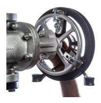
4. Center the chainwheel and tighten the nuts securely.
