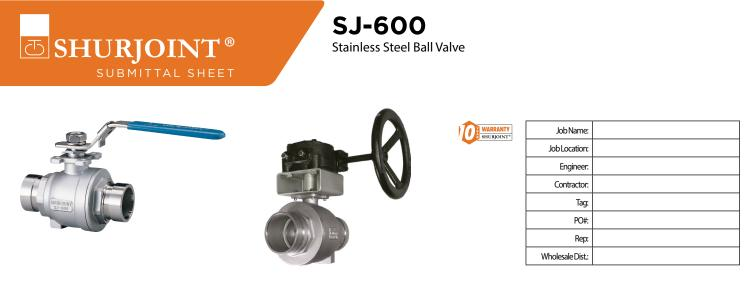
The Model SJ-600L is a stainless steel, grooved-end, two-piece, full port ball valve designed and tested in conformance with MSS SP-110 and SP-72. The lever handle is equipped with tamper resistant locking holes. The SJ-600L is comprised of a stainless steel body and end cap, virgin TFE seats and stainless steel trim. The valve is supplied standard in CF8M (316).
