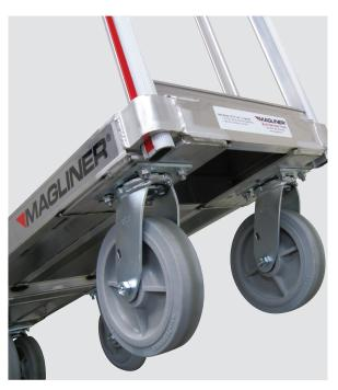
Robotically welded five-box aluminum construction optimized for over-the-road payload.
