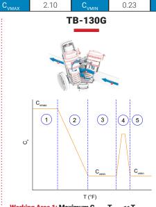
Working Area 1: Maximum C<sub>vmax</sub>, T<sub>water</sub> << T<sub>desiredrecirc</sub> In this temperature range, the valve is completely open and a spring is balancing the thermostatic cartridge
