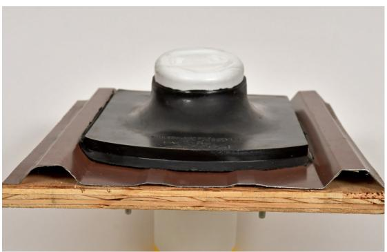
The Kozy Kollar seal if formed by the compression of the Main Seal and roof material between the Main Frame of the Kozy Kollar and the substrate of the roof. If there is not a solid substrate were the Kozy Kollar will be installed a piece of 3/4 plywood must be installed under the metal roof. The plywood should be at least the size of the Kozy Kollar.
