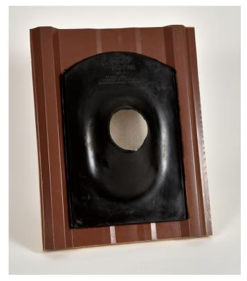
The Kozy Kollar will also work on a metal, rolled or rubber roofs. To insure a tight seal the Kozy must be set on a flat section on the roof. The area should large enough to accommodate the Kollar, 8" wide for the PV-3 or PV-2 and 9.25" for the PV-4 and EV-4.
