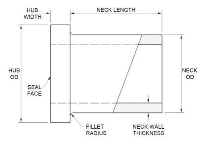
FIG. 3 POLYETHYLENE FLANGE ADAPTER GEOMETRY
