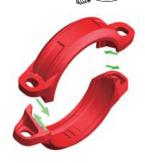
**T&G design:** The T&G (tongue & groove) mechanism provides a mechanical and frictional interlock resulting in a rigid joint which reduces undesired angular movement. ARGCO precision casting techniques allow the coupling segments to meet metal-to-metal when installed on properly grooved pipe.
