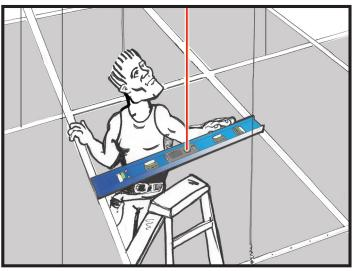
•Simply measure sprinkler drop to projected laser, and subtract your takeout
