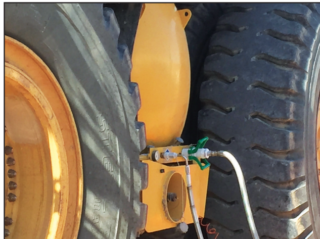
LNG fueling application on off-highway mining truck
