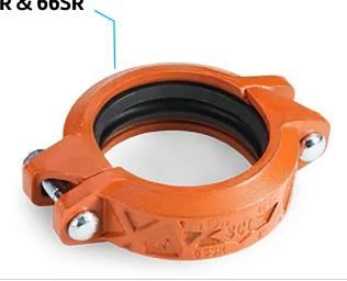
Figure 65SR & 66SR Standard Weight Rigid couplings are designed for use in piping systems when rigid piping connections are desired. The angle-pad design allows the coupling housing to slide when tightened. This provides offset clamping that creates a rigid joint resistant to flexural and torsional loads.
