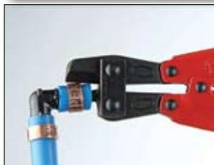
1. Cut off PEX tube close to the fitting. Insert small jaw inside fitting and fully close handles, forcing cutter through crimp ring.
