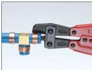
RINGCRUSHER cuts crimp rings off fittings and expands crimped tubing for easy removal. It only takes a few seconds. New heavy-duty design cuts crimp rings on 1/2", 3/4" and 1" copper, brass and poly alloy/plastic fittings and tube without damage to inside fittings. Stop wasting time using a hacksaw or torch, and stop throwing away expensive PEX fittings.
