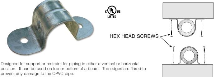
It is easily attached using two #10 x 1" hex head self-threading screws (supplied).
