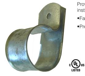
Provides support for CPVC piping in fire sprinkler systems installed per NFPA 13, 13R and 13D.
