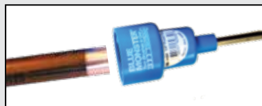
Fully retract fitting brush into the housing to clean O.D. of copper tube.
