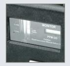
An Easy-View Window provides visibility to the displays without having to open the case. The flow gauge indicates active air sampling, LED lights show Barricade CO Monitor status, and the LCD display indicates the level of CO present in the air.
