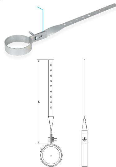
Size Range: 11/2" through 4" NPS Material: Carbon steel Finish: Electro-Galvanized Service: Pipe hanger or restraint for DWV pipe.
